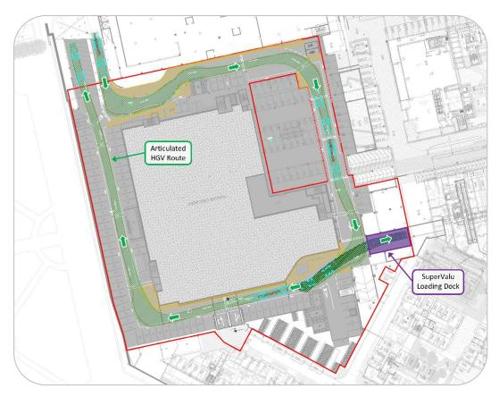
Figure 4 – HGV servicing of existing SuperValu retail unit
